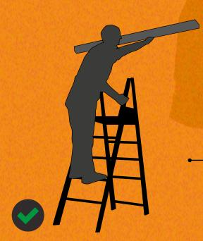
Make sure you always have a secure place to hold at the correct height by working no higher that the 3rd rung from the top
